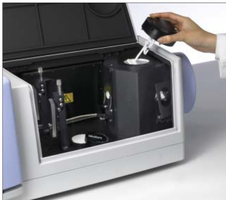
Figure 3. The 150 mm integrating sphere with sampling module lid open.
